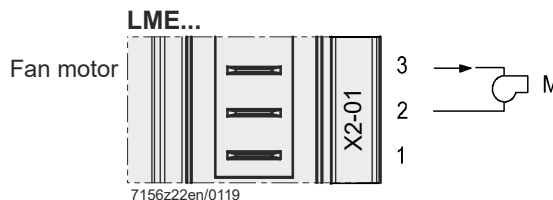
Figure 18: Fan motor terminal X2-01
