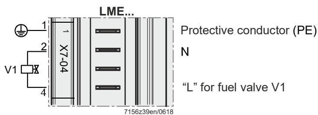
Figure 40: Fuel valve V1 terminal X7-04
