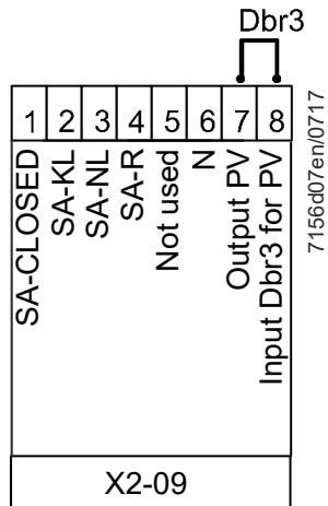
Figure 34: Connection diagram example 5: for LME75.000Ax with PME75.831Ax without actuator
