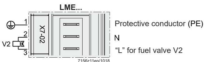
Figure 42: Fuel valve V2 terminal X7-02
