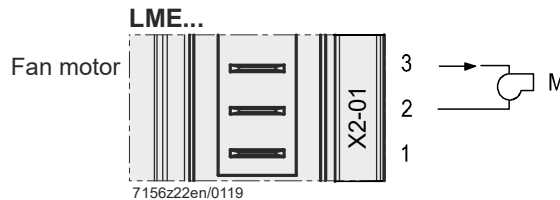
Figure 16: Fan motor terminal X2-01
