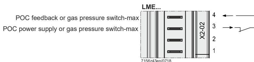
Figure 8: POC or gas pressure switch-max terminal X2-02
