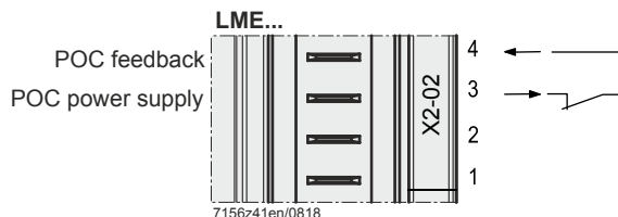
Figure 19: POC function input terminal X2-02
