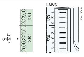
Measuring circuit for detector current measurement
