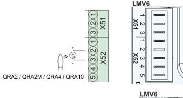
Measuring circuit for detector current measurement
