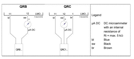
As an alternative to detector current measurement, the Interface OCI400 with PC software ACS410 can be used. In that case, the DC microammeter is not required.
